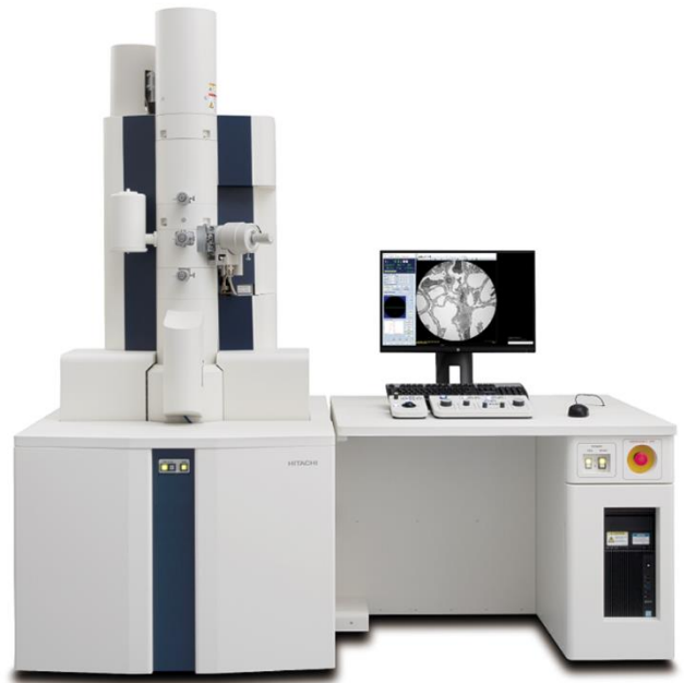
Figure 1 – The ViroTEM system is a compact TEM-based analysis tool designed for simple operation but with powerful functionality
